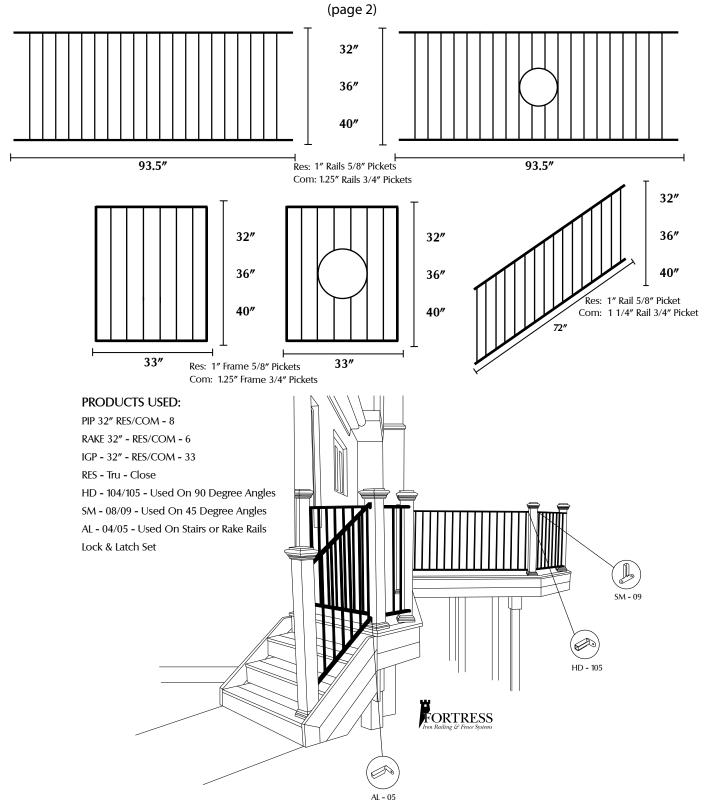
32" panels installed to build 36" railing set for 8" on center when used with 2" x 2" post. All panels mounted with brackets for easy installation.
